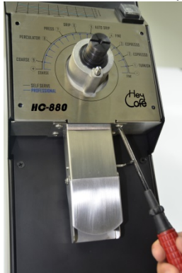
Step 1 -remove chute
