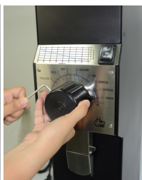
Fig 8.2 loosen the securing screws
